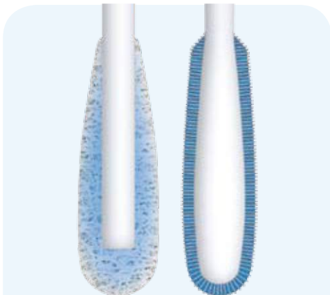
Traditional Fiber Swabs consist of Fiber Wads FLOQSwabs™ have no inside
