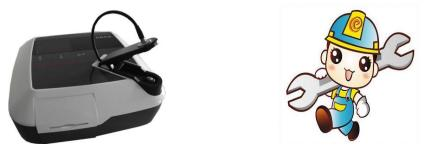
For MaestroNano, the only possibility needed calibration is from Xe lamp. Xe lamp is responsible to emit every wavelength we want to measure, having lifetime more than 1 million tests (equal to 10 years roundly). Xe lamps can work normally for long time but its intensity may become weaker after 3~5 years operation. At that time, Maestrogen will update calculation formula to fit this change. So, MaestroNano still needs some calibrations, but only once per 3~5 years.
