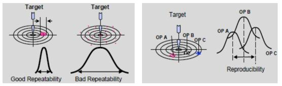
Repeatability is the ability of the same gauge to give consistent measurement readings no matter how many times the same operator of the gauge repeats the measurement process. Reproducibility, on the other hand, is the ability of the same gage to give consistent measurement readings regardless of who performs the measurements. The evaluation of a gage's reproducibility, therefore, requires measurement readings to be acquired by different operators under the same conditions.
