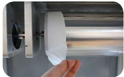
Membrane Layer collected on the cylinder collector
