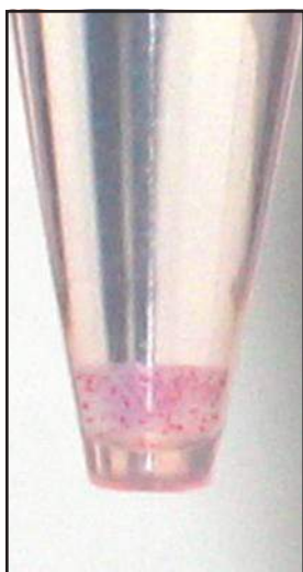
Visible Agarose Beads Provided in the Small GTPase Activation Assays. Beads are easy to visualize, making it easier to avoid potential loss during washes and aspirations.
