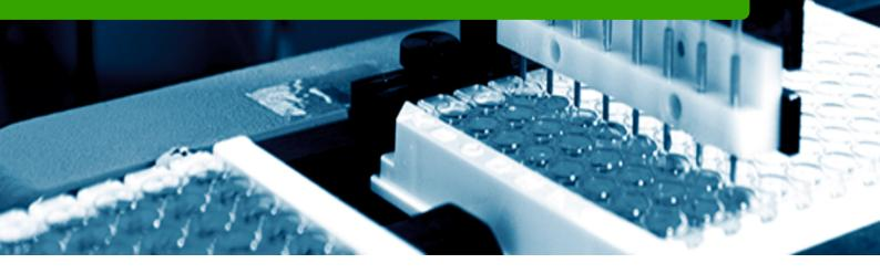
The 300 DMC Microplate Dispensing System is the best choice for highly accurate, precise and reproducable Microplate dispensing applications in a production environment. Up to 4 DMC's can be configured to a single dispense conveyor, resulting in a through-put of over 1,000 dispensed microplates per hour, while maintaining CV below 2%.
